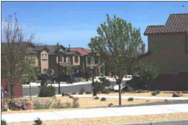
Integrating pedestrian connections at the bulb of a cul-de-sac promotes a walkable environment.
